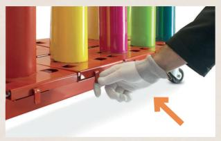
Lock levice to prevent rolls from falling out during transport
